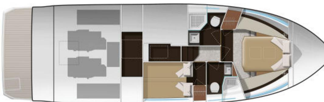
The Velasco 43F has two heads with separate shower stalls, which is not always a given on a boat that's less than 45' (13.7 m) long. We consider this one of the important features of the boat.
