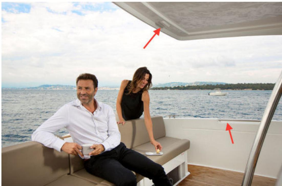
In the cockpit, the LED lights are part of the “Premiere” upgrade package. Note the handrail recessed into the gunwale for security.
