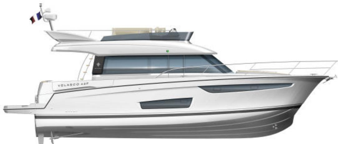
The most important difference between the Velasco 43 and the new Velasco 43F is the rake of the forward windshield and the absence of skylights in the forward, flybridge cowling. Also, the radar mast has been moved aft and minimized and fins have been added to balance the overall look of the boat's top hamper and to support the radar arch.
