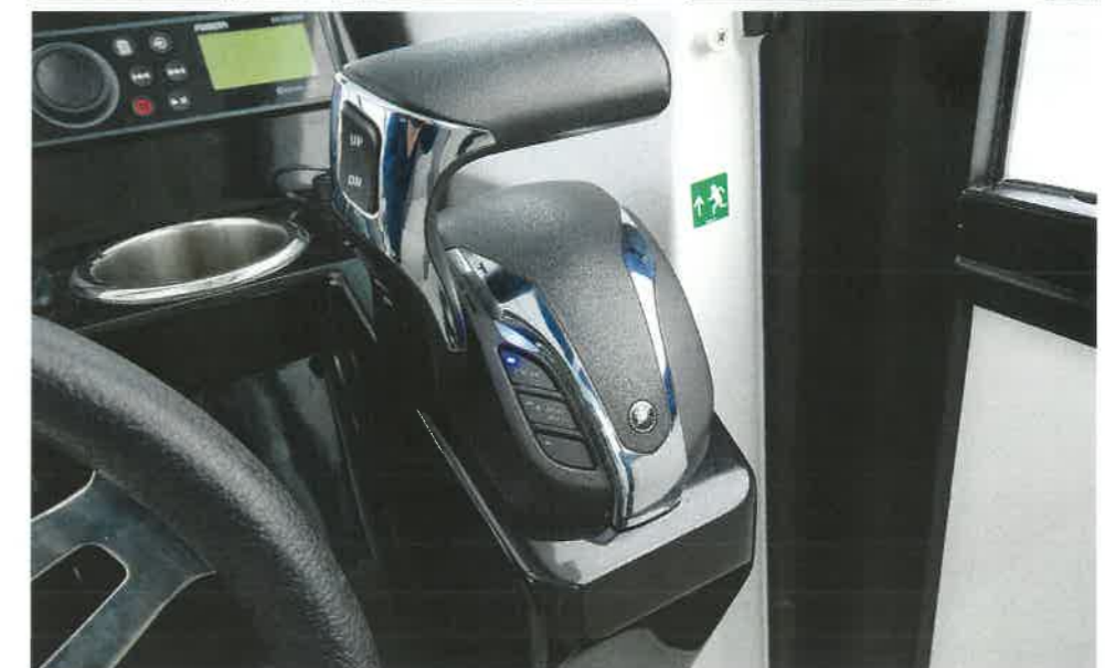
Right 1: Bow thruster is fitted, as is a Zipwake trim system (UK Dealer: Hypromarine) 2: Excellent Yamaha fly-by-wire controls are precise.
