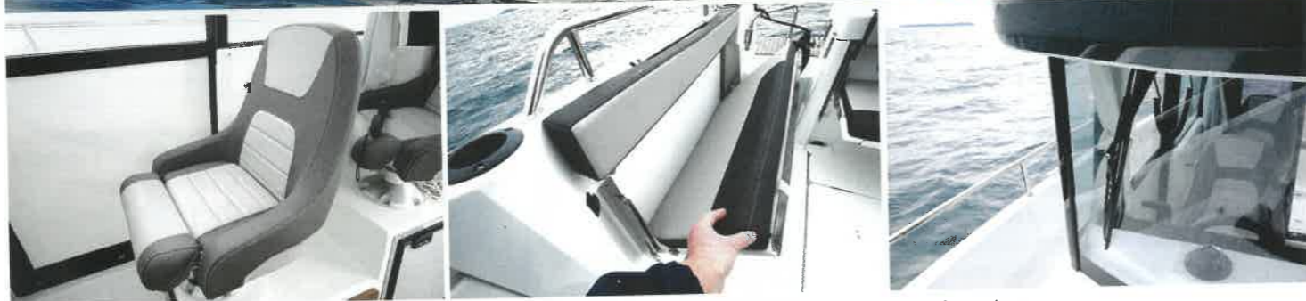
1: Grippy seats with flip-up bolsters. 2: Trademark Jeanneau stowaway seats in the cockpit. 3: Curvy screen has wipers.
